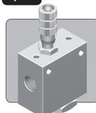
The CMF50 is a 1/2" nominal bore metering valve with a reverse free-flow check function. It provides metered flow in one direction, and free flow in the opposite direction, ideal for uni-directional speed control of a cylinder or actuator.
